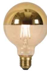
1101002700 LED bulb globe filament top mirror gold Ø9.5xh.14cm, E27/3.5W dimmable, 250Lm/2300K
